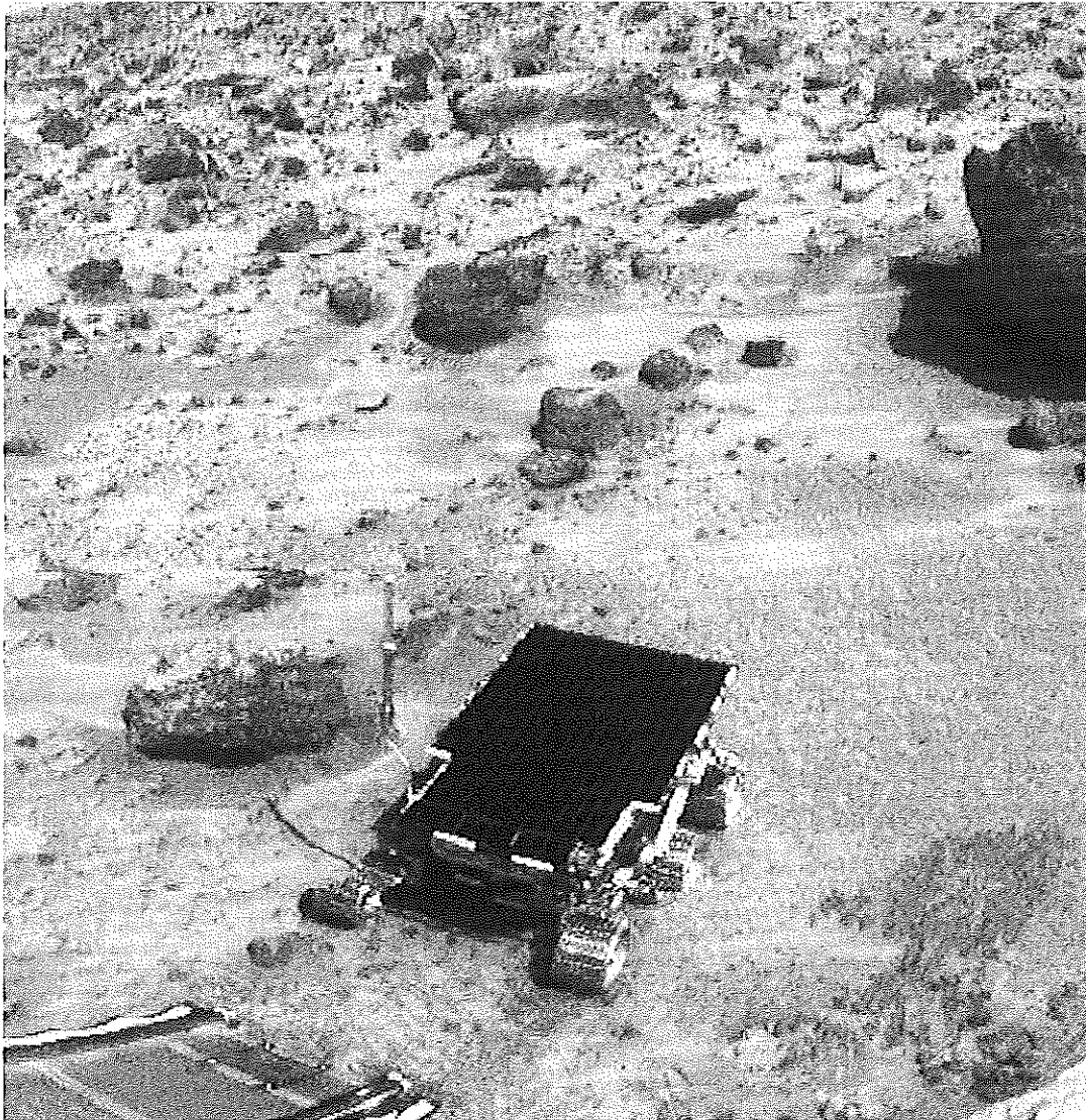
Mars Pathfinder's twenty-five-inch-long rover Sojourner was the first vehicle of its kind to be landed on the surface of an extraterrestrial body. Here, it has been photographed by its base station alongside a rock dubbed "Barnacle Bill." A larger rock named "Yogi" awaits exploration at the upper right. A portion of the ramp leading to the surface from the base station appears at the lower left. JPL/NASA
