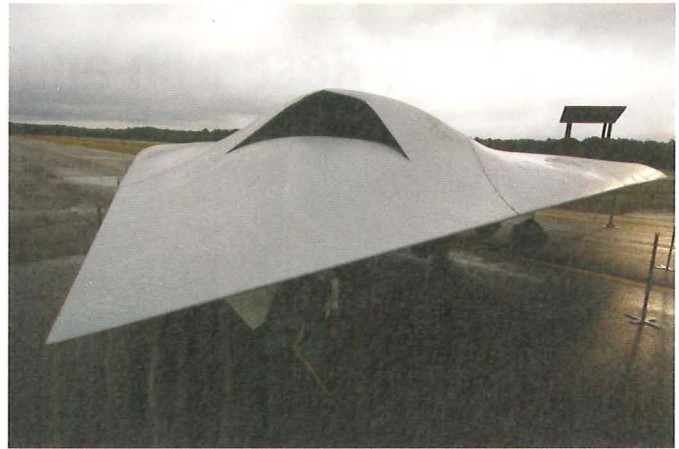
A demonstration model of a future stealthy robot strike aircraft. They would operate from an aircraft carrier, and be the first wave in a strike to take out enemy air defenses prior to sending in manned aircraft. Such aircraft might someday engage in air-to-air warfare with their enemy robotic counterparts.
