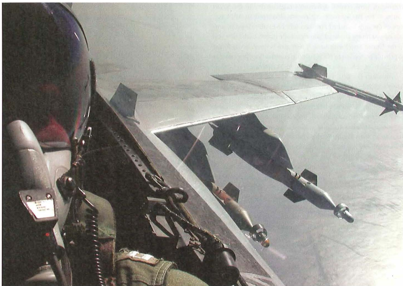
Two 500-pound laser-guided "smart bombs" and a Sidewinder missile on the wing of a F/A-18 Hornet.
