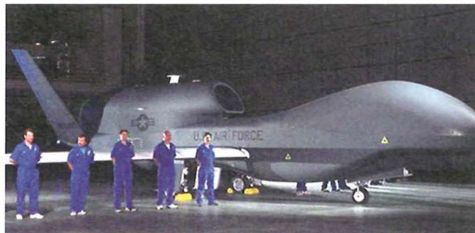
The Global Hawk UAV is a large Air Force endurance drone, able to cruise at 400 miles per hour for thirty-five hours. It can scan an area the size of the state of Illinois in just twenty-four hours. (Air Force photo)
