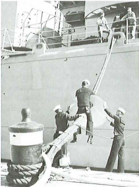
When a ship is secured to a pier, the mooring lines are usually doubled up, as shown here. Then light line is used to bind the parts together, and conical rat guards are put in place so that rats and mice cannot crawl up the lines onto the ship.
