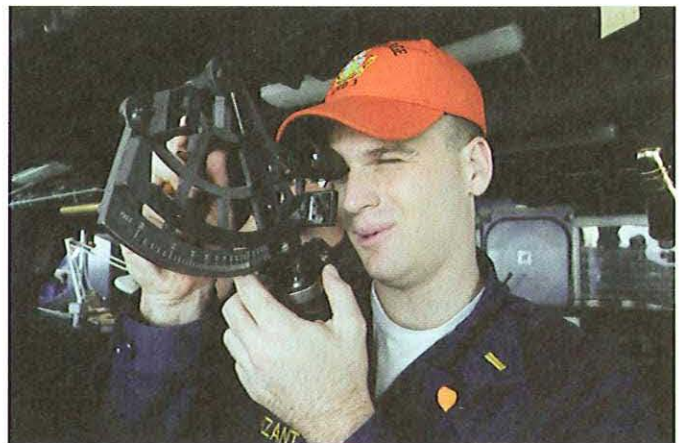
A watch officer measures the distance to another ship with a Brandon sextant-type stadimeter. The stadimeter measures the distance to an object of known height, such as the masthead of a ship. (Emmitt Hawkes)
