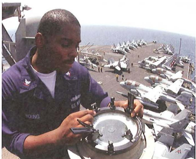
A quartermaster on the aircraft carrier USS John F. Kennedy (CV 67) uses a bearing circle to obtain a true bearing to an object. (Anthony Riddle)
