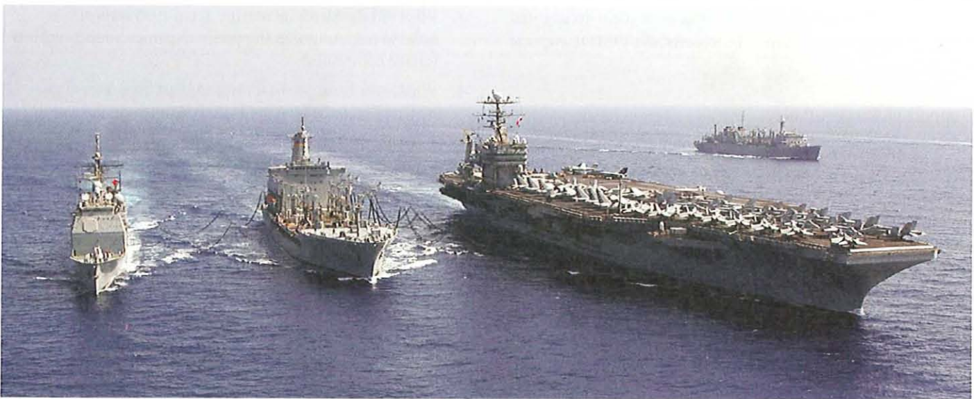
An underway replenishment operation with the oiler USNS Leroy Grumman simultaneously refueling a Navy aircraft carrier and a destroyer. The replenishment ship USNS Supply is in the background.
