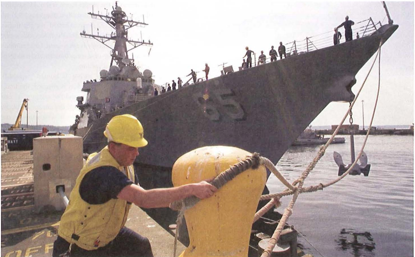
A boatswain's mate passes the eye of a second bow line from a Navy destroyer over a bollard on a pier. Note the stockless anchor dangling from the hawsepipe, ready to be let go if the ship had difficulty while maneuvering into its berth. (Douglas Morrison)
