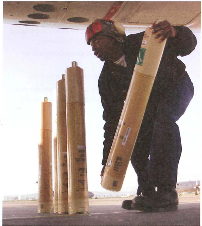
An aviation ordnanceman loads disposable radio sonobuoys into a P-3 Orion patrol aircraft. The sonobuoys can be dropped on the water around a suspected submerged submarine, allowing an operator on the aircraft to track its movements. (John Collins)
