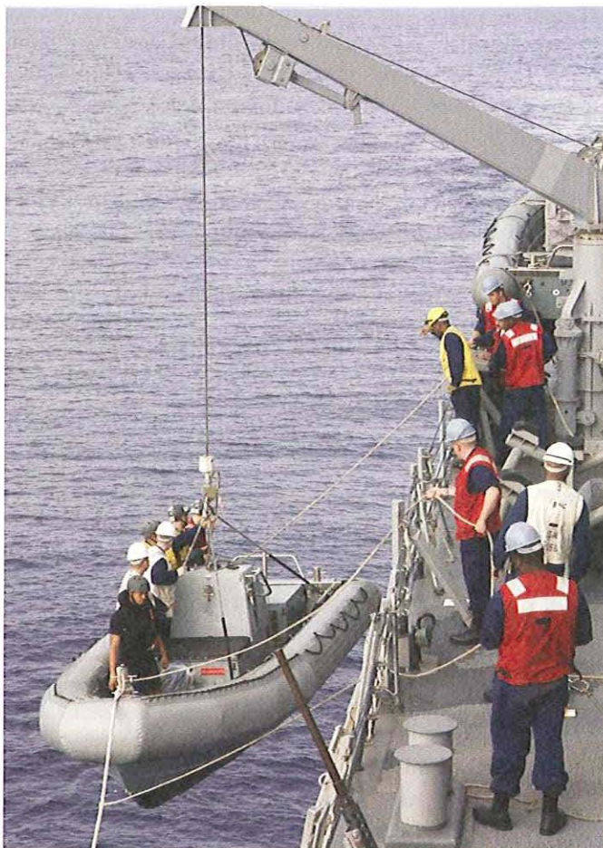
Rigid hull inflatable boats (RHIBs) have become the workhorses among the small craft of the fleet, doing duty as lifeboats, personnel boats, fast patrol craft, and utility boats.
