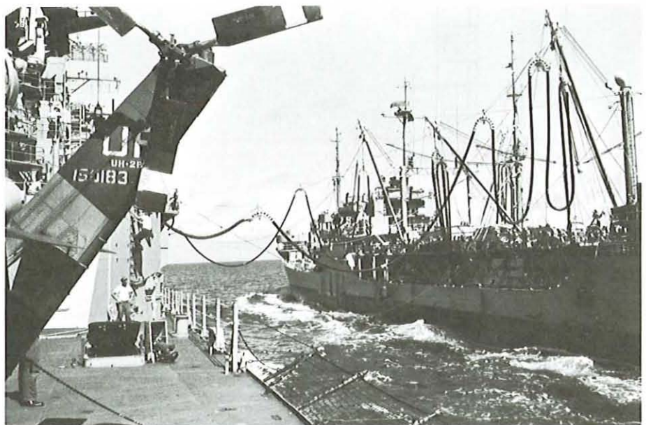
Several booms and their rigging are shown in use by this oiler during an underway replenishment of another ship alongside.
