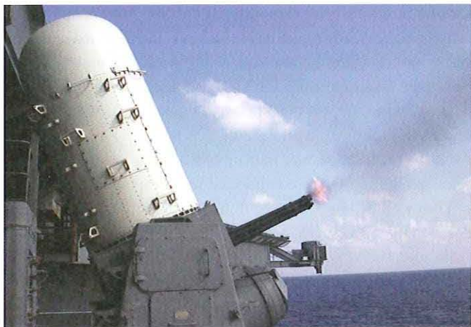
The Phalanx close-in weapon system is a 20-mm fully automatic gun system designed as a ship's last-ditch weapon against antiship cruise missiles. The gun is a six-barrel Vulcan Gatling gun capable of firing three thousand rounds per minute to a range of about 1 mile. (Philip McDaniel)
