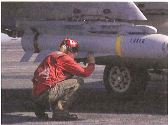
An aviation ordnanceman arms a Maverick missile on a F/A-18 Hornet. (Gretchen Roth)
